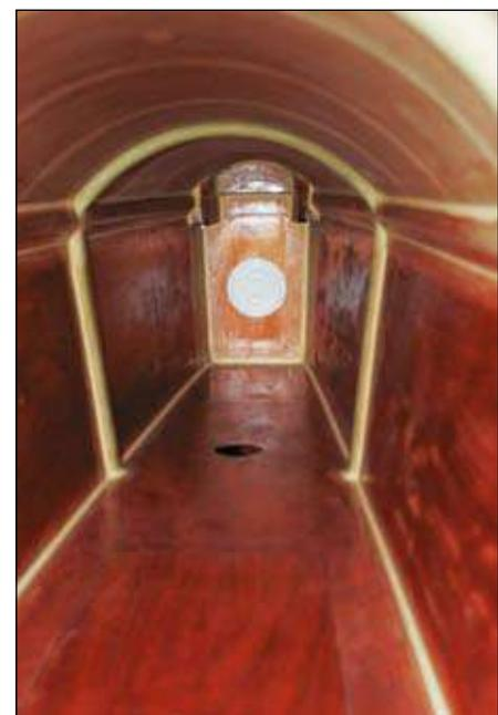
John Tetzlaff built *Attitude* using the compounded plywood construction method – see explanation page 50.
