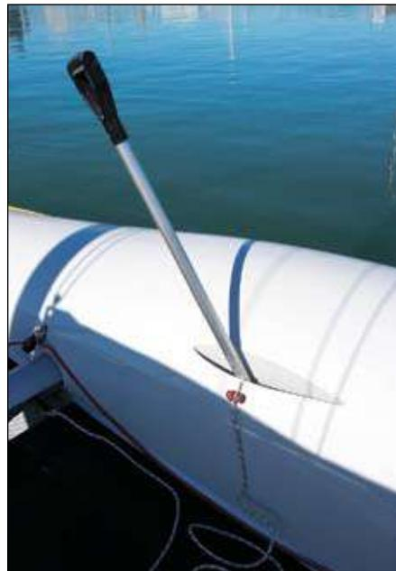
A central pod supports the outboard motor and stiffens the main beam. Spade handles raise and lower the daggerboards.
