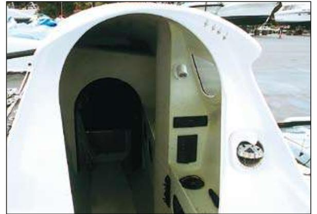
**ABOVE CENTRE:** The outboard pod allows maximum clearance with the outboard up and maximum prop depth when outboard is down.
